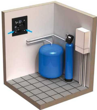
OV fan boiler room ventilation example.
